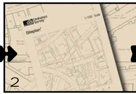
2 A site location plan (scale 1:1250 or 1:2500). Outline the application area in red. If you own any adjoining land outline that in blue. Show some of the surrounding area and the direction of north. The site location plan should be drawn from a recent Ordnance Survey map on an A4 sheet (the same size as this Guide). Copies can be bought quite cheaply from a map shop.
